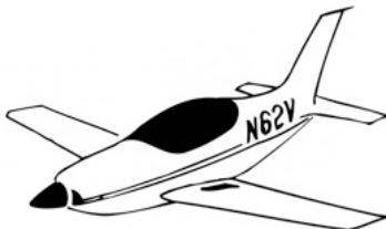
Questair Venture: W = 8,000 \text{ N} , S = 6.76 \text{ m}^2 , b = 8.40 \text{ m} , P = 224 \text{ kW} (300 hp).
