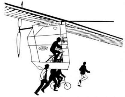
Gossamer Albatross: W = 940 \text{ N} , S = 70 \text{ m}^2 , b = 29 \text{ m} .
