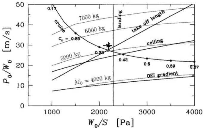
There is still one further problem with the analysis: we assumed  $W_{fuel}/W_0 = 0.1712$ , a constant, regardless of where we are on the plot. We already know that for a fixed cruise speed, changing  $W_0/S$  will change  $C_L$ , hence  $C_L/C_D$ , and so, fuel consumption.
