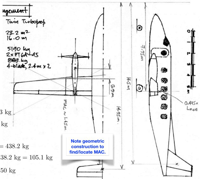
For this type of layout we can choose to let the engines move fore and aft with the wing.
