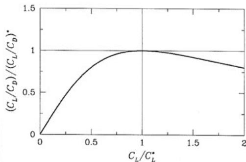
$$\begin{aligned} L/D &= \frac{1}{C_D/C_L + K_C} \\ &= \frac{1}{0.02/0.3767 + 0.036 \times 0.3767} \\ &= 15.0. \quad (\text{cf } (L/D)^* = 18.6). \end{aligned}$$
