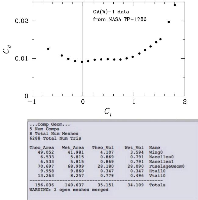
These are the data for the 17% thick section used at the wing root.
