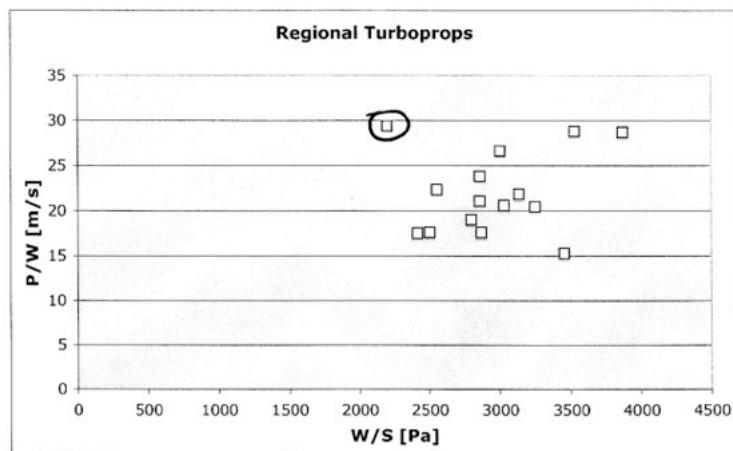
We see our initial sizing places our design at a lower wing loading and higher power loading than all the other designs.
