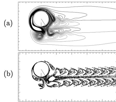
FIG. 1. Flow produced by cylinder with combined oscillatory translation and rotation: (a) instantaneous vorticity contours; (b) fluid particle transport. The cylinder is at its maximum vertical position and most negative angular displacement at the instant shown. The rest position of the cylinder is indicated by cross-hairs, and the radial line shows the rotational displacement of the cylinder.
