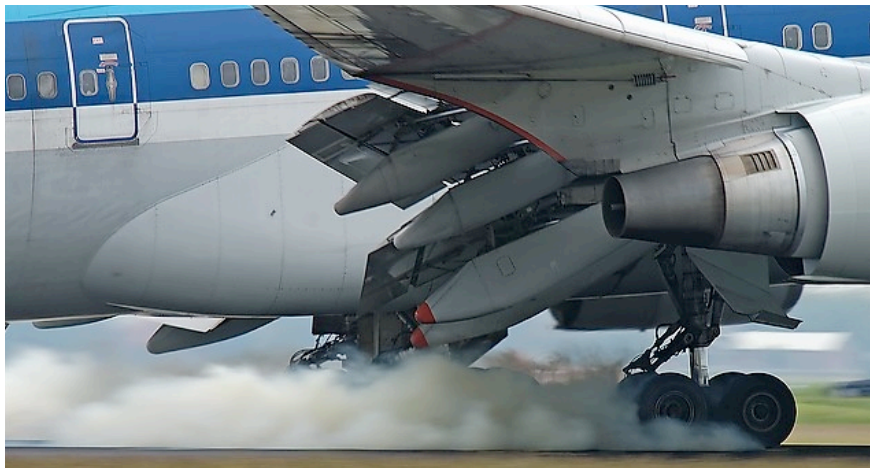
747 high-lift system at touchdown.
