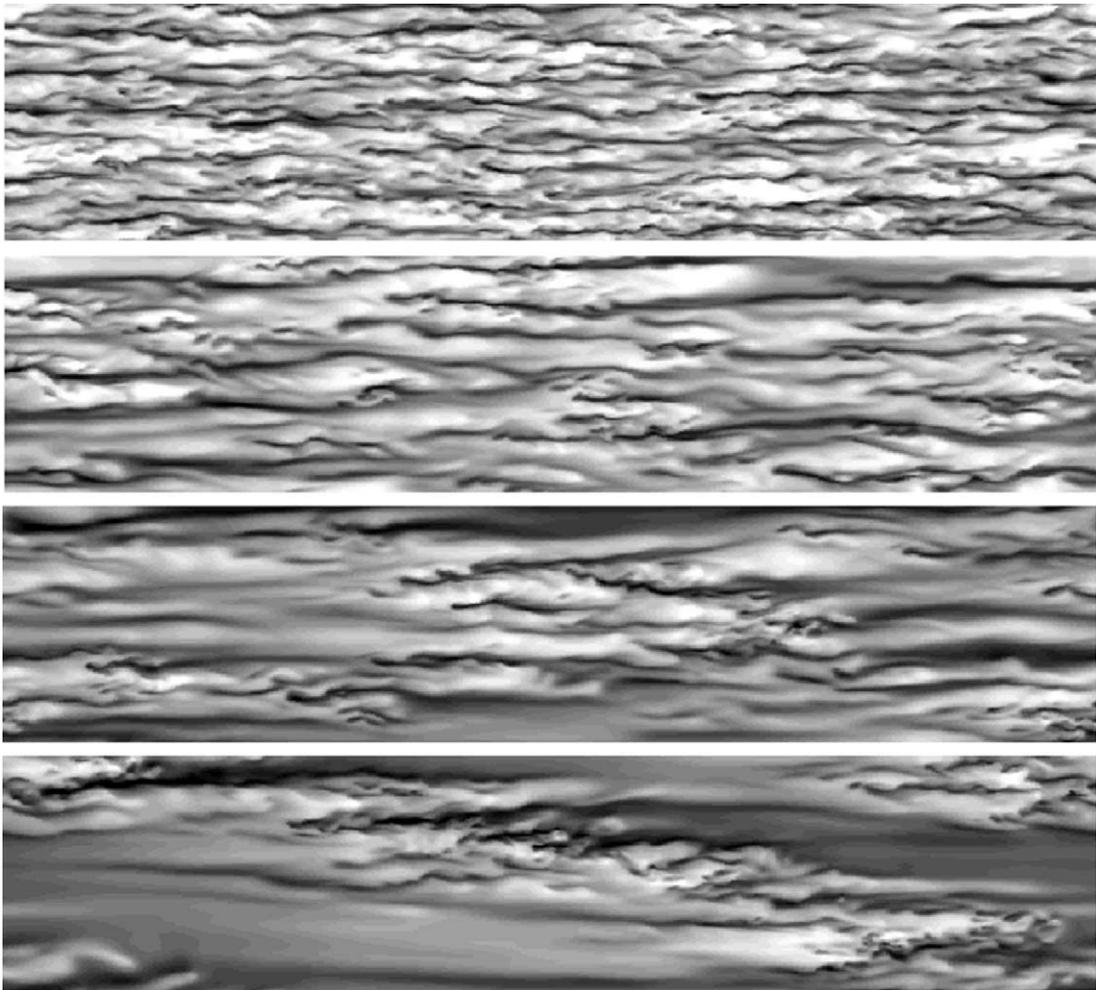
Fig. 10. Predicted axial velocity at  $y^+ \approx 20$  for  $Re_G = 7500$ . From top to bottom, Newtonian, PL ( $n = 0.6$ ,  $\tau_Y = 0$ ), HB1 ( $n = 0.6$ ,  $\tau_Y = 0.1\tau_w$ ), HB2 ( $n = 0.6$ ,  $\tau_Y = 0.5\tau_w$ ). The pipe surface has been rolled flat and the flow is from left to right. White represents high velocity and black low.
