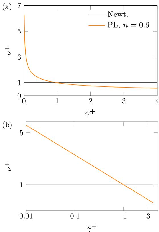
FIG. 2. Viscosity rheograms plotted for Newtonian and PL fluids on (a) lin-lin and (b) log-log axes.
