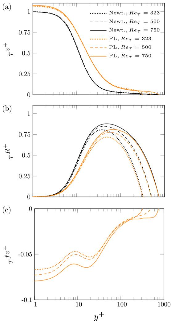
FIG. 15. Profiles of the (a) mean viscous stress  $\tau^{v^+}$ , (b) Reynolds shear stress  $\tau^{R^+}$ , and (c) turbulent viscous stress  $\tau^{fv^+}$  plotted for Newtonian and PL fluids at different  $Re_\tau$ .
