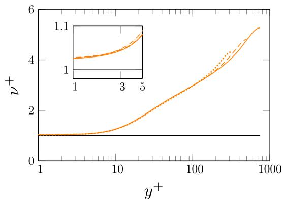
FIG. 12. Profiles of the normalized mean viscosity plotted for PL fluid at different  $Re_\tau$ . For the line legend see Fig. 9.
