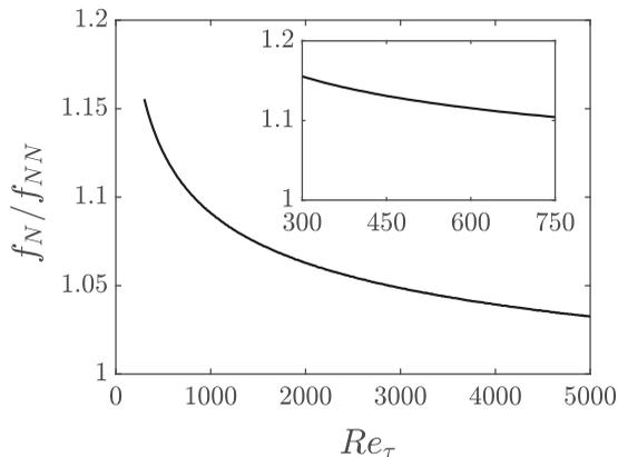
FIG. 14. Ratio of friction factors for Newtonian and PL fluids obtained from the correlation (13) plotted against  $Re_\tau$  with the inset showing a closer look in the  $Re_\tau$  range considered in this study.
