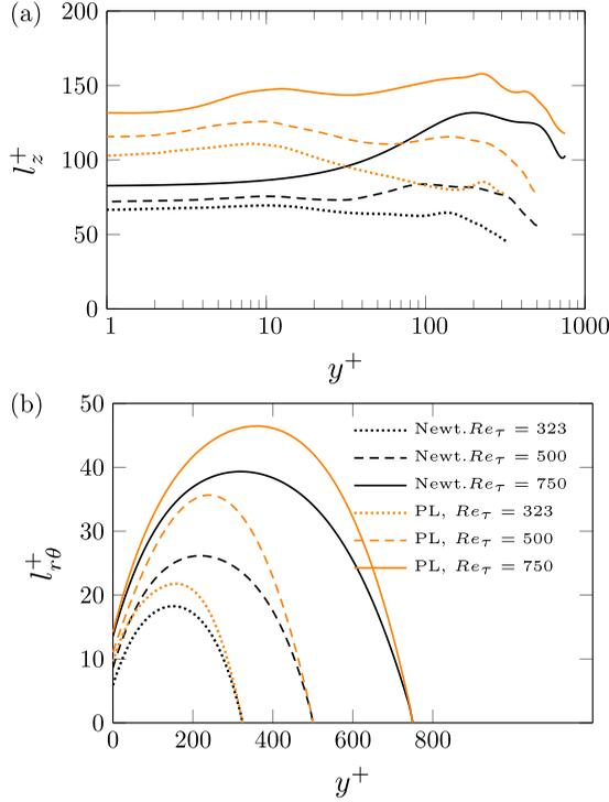
FIG. 8. (a) Streamwise and (b) azimuthal integral length scales of axial velocity fluctuations plotted as a function of  $y^+$ .
