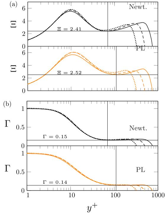
FIG. 10. The (a) log-law and (b) power-law indicator functions for Newtonian and PL fluids. Vertical lines show the location where the labeled values are read.
