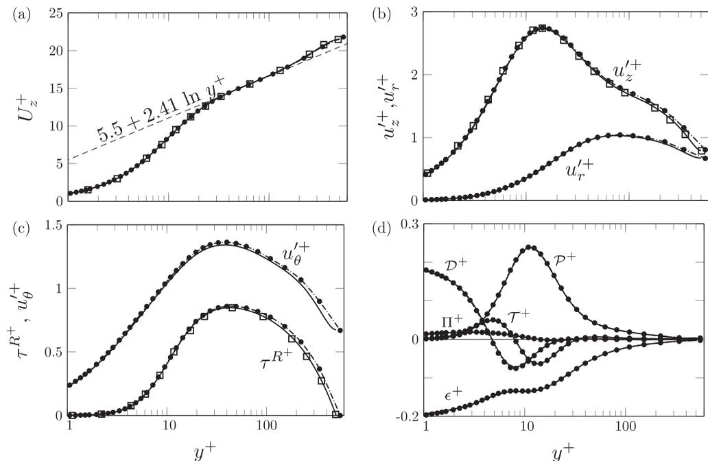
FIG. 5. Inner-scaled statistical profiles from DNS of Newtonian fluid at  $Re_\tau = 500$  (solid line), compared to DNS results of El Khoury *et al.* [20] (closed circles,  $Re_\tau = 550$ ) and Chin [23] (open squares,  $Re_\tau = 500$ ): (a) mean axial velocity, (b) rms of axial and radial velocity fluctuations, (c) Reynolds shear stress and azimuthal velocity fluctuations, and (d) turbulent kinetic energy budget.
