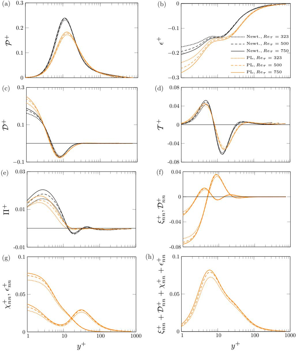
FIG. 19. Profiles of the turbulent kinetic energy budget terms [see Eq. (A2)] plotted for Newtonian (black lines) and PL fluids (orange lines) at different  $Re_\tau$ .
