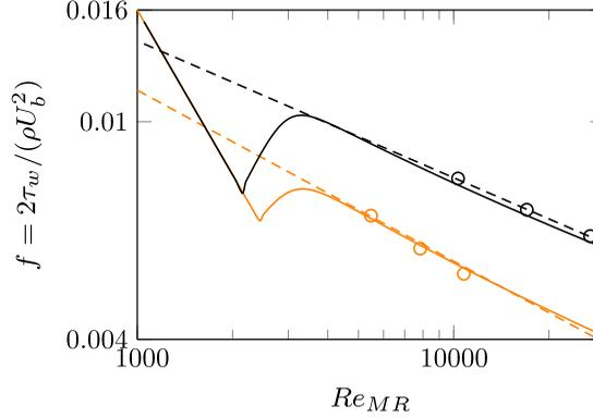
FIG. 13. Comparison of the friction factor obtained via DNS (circles) and those of the Dodge-Metzner correlation (solid lines) and the Anbarlooei *et al.* correlation (dashed lines) for Newtonian (black lines) and PL fluids (orange lines).
