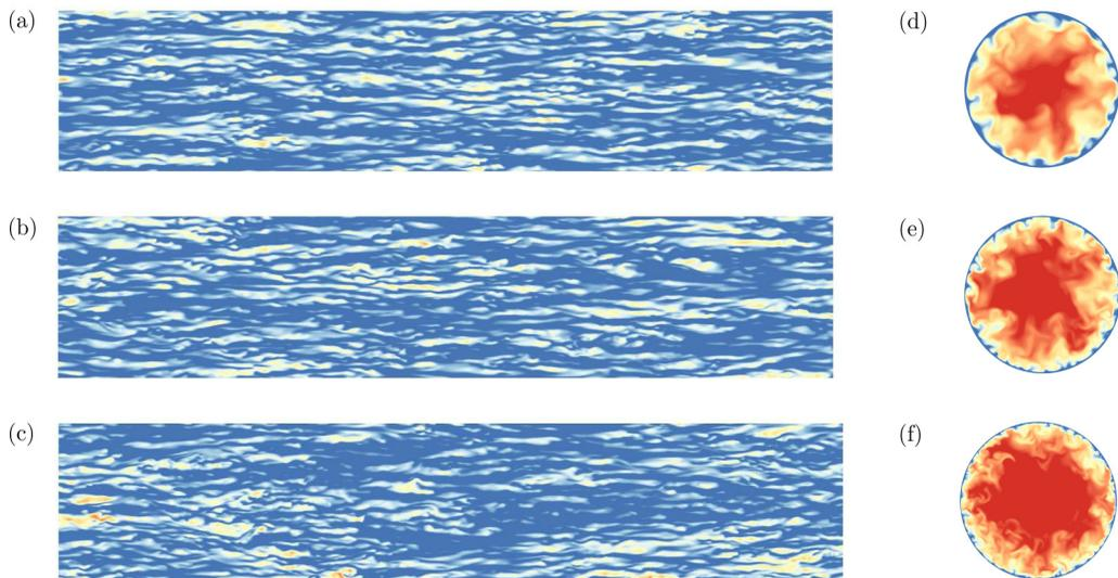
FIG. 6. Contours of inner-scaled instantaneous axial velocity  $u_z^+$  plotted in (a)–(c) inner coordinates on a developed cylindrical surface  $z^+ - r\theta^+$  at  $y^+ = 10$  and (d)–(f) outer coordinates on a cross section for a Newtonian fluid at (from top to bottom)  $Re_\tau = 323, 500,$  and  $750$ . For (a)–(c), the flow is from left to right and the region is 7000 wall units long and 1600 wall units wide. The contour levels vary from blue to red with the values 8–20.
