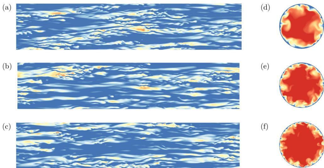
FIG. 7. Contours of inner-scaled instantaneous axial velocity  $u_z^+$  plotted in (a)–(c) inner coordinates on a developed cylindrical surface  $z^+ - r\theta^+$  at  $y^+ = 10$  and (d)–(f) outer coordinates on a cross section for PL fluid at (from top to bottom)  $Re_\tau = 323, 500,$  and  $750$ . For (a)–(c), the flow is from left to right and the region is 7000 wall units long and 1600 wall units wide. The contour levels vary from blue to red with the values 8–20.
