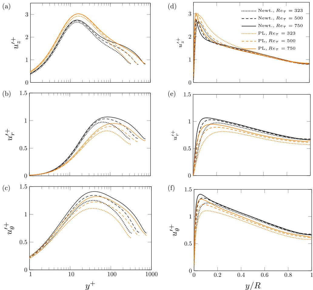
FIG. 16. Profiles of turbulence intensities plotted as a function of (a)–(c)  $y^+$  and (d)–(f)  $y/R$  for Newtonian and PL fluids at different  $Re_\tau$ .
