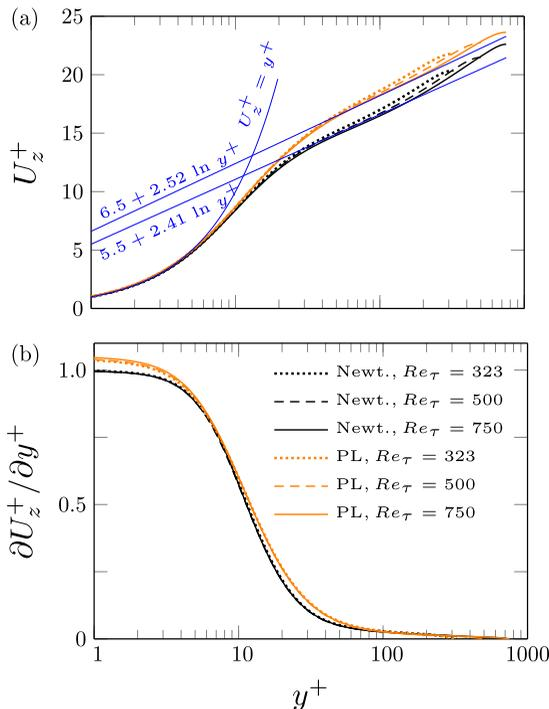
FIG. 9. Profiles of the inner-scaled (a) mean axial velocity and (b) mean axial velocity gradient plotted for Newtonian (black lines) and PL fluids (orange lines). Blue lines in (a) show the law of the wall with the slope parameter determined in Fig. 10 (a) for  $Re_\tau = 750$ .
