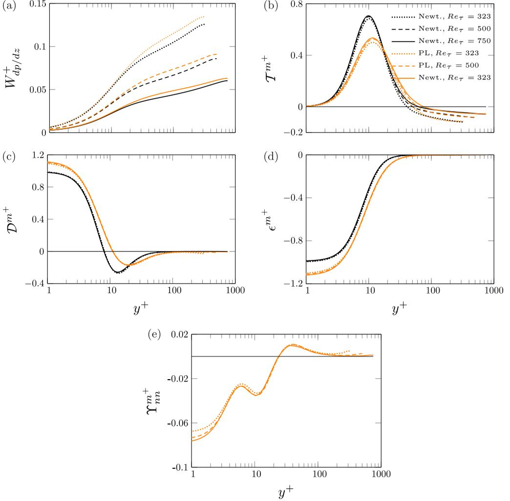
FIG. 18. Profiles of the terms which appear only in the mean flow kinetic energy budget (A1) plotted for Newtonian (black lines) and PL fluids (orange lines).
