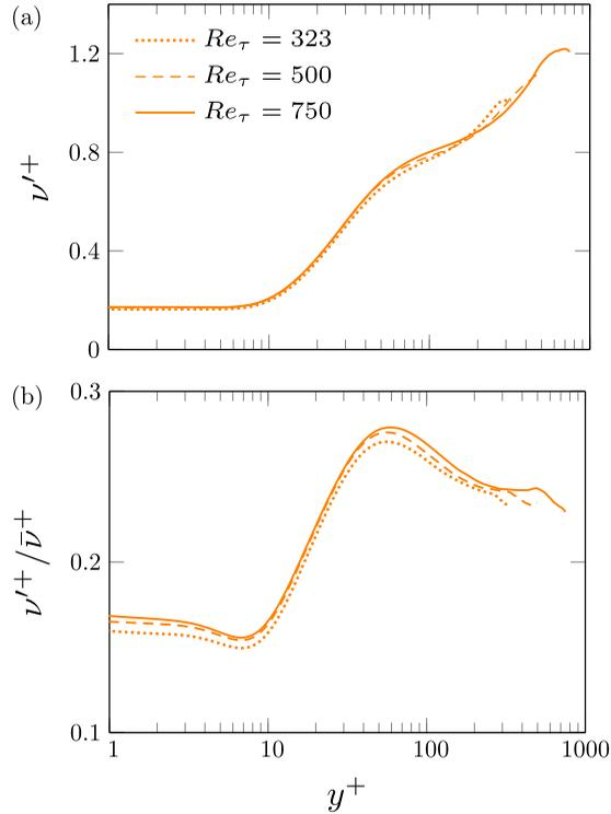
FIG. 17. Profiles of the rms viscosity fluctuations normalized by (a) the nominal wall viscosity and (b) the local mean viscosity plotted for PL fluid at different  $Re_\tau$ .
