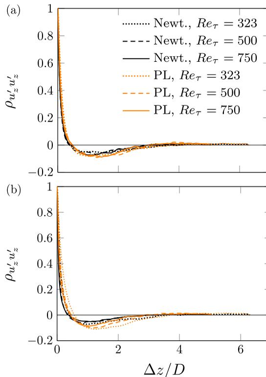
FIG. 3. Two-point correlation coefficient of axial velocity fluctuations plotted as a function of separation distance  $\Delta z/D$  at (a)  $r/D = 0.35$  and (b)  $r/D = 0.48$ .
