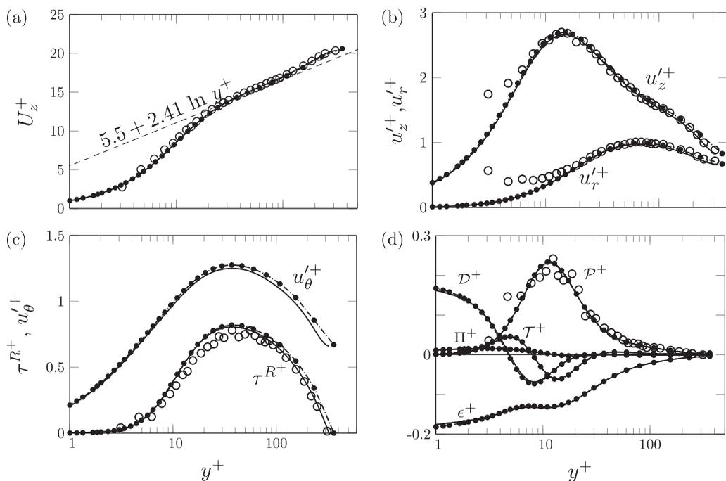
FIG. 4. Inner-scaled statistical profiles from DNS of Newtonian fluid at  $\text{Re}_\tau = 323$  (solid lines), compared to experimental results of den Toonder and Nieuwstadt [22] (open circles,  $\text{Re}_\tau = 314$ ) and DNS results of El Khoury *et al.* [20] (closed circles,  $\text{Re}_\tau = 360$ ): (a) mean axial velocity, (b) rms of axial and radial velocity fluctuations, (c) Reynolds shear stress and azimuthal velocity fluctuations, and (d) turbulent kinetic energy budget.
